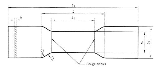
$b_1$  Width of narrow parallel-sided portion: 25,4 mm  $\pm$  0,1 mm
