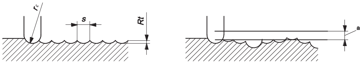
a) Theoretical finish for ideal cutting with zero asynchronous error motion b) Effect of asynchronous error motion on peak-to-valley roughness with ideal cutting
