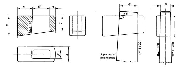
1) The dimensions E and F, depending on the material of which the picker is made, should be chosen so that, when the picker is mounted, it fits tightly on the picking stick.
