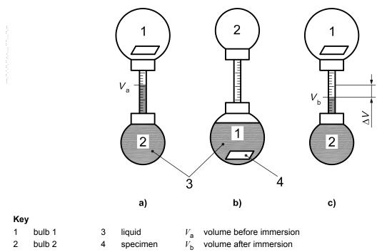
Figure 1 — Specimen-immersion apparatus
