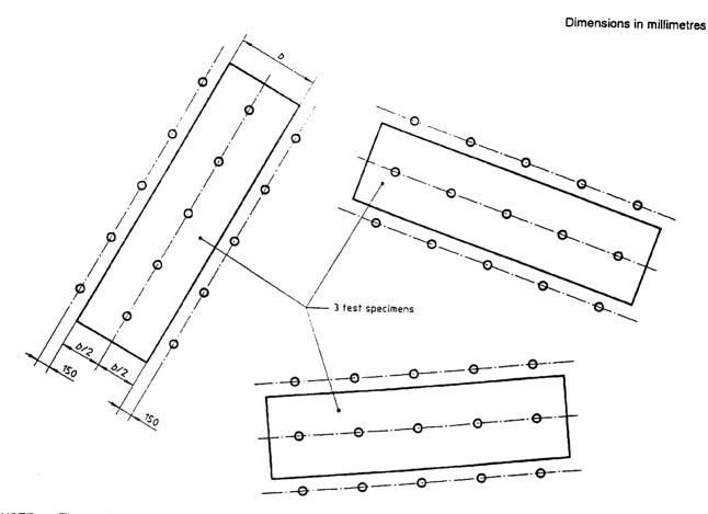
NOTE — The small circles mark the position where the hammers of the tapping machine should strike the bare floor or the test specimens respectively.
