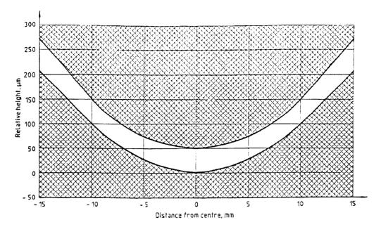
NOTE The relative height at the centre can be chosen freely within 0  $\mu m$  to 50  $\mu m$  to make the curvature of the hammer head fit within the tolerance limit.
