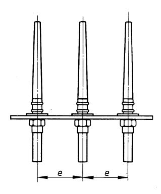
The spindle gauge  $\boldsymbol{e}$  is the distance between the axes of two adjoining spindles.
