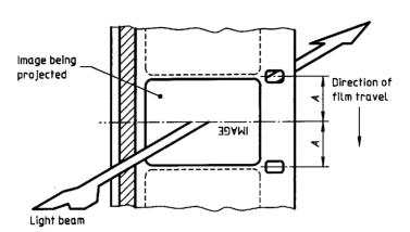
The film is shown as seen from the light source in the projector looking towards the projector lens.
