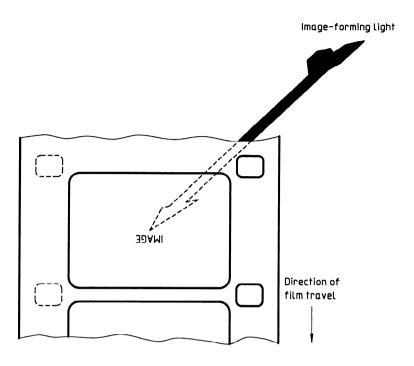
The film is shown as seen from inside the camera, looking towards the lens with the photographic layer away from the observer, towards the lens.
