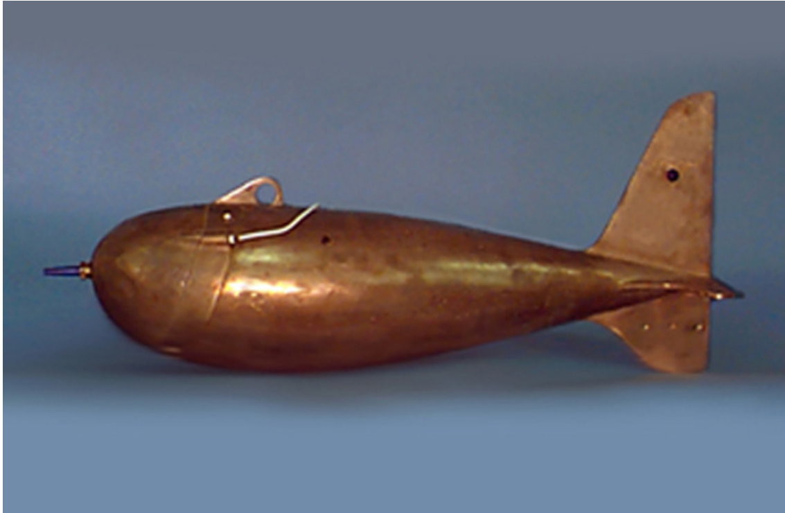
Figure 6 — US P-61-A1 suspended-sediment sampler developed by the Federal Interagency Sedimentation Project in the United States
