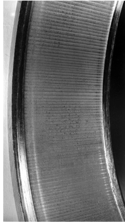
Figure 27 — False brinelling — Fluting on outer ring of tapered roller bearing
