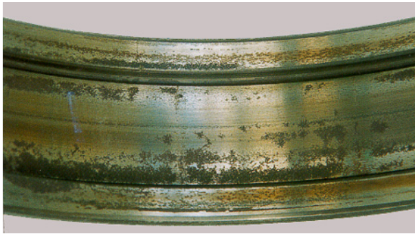
Figure 22 — Corrosion on roller bearing outer ring
