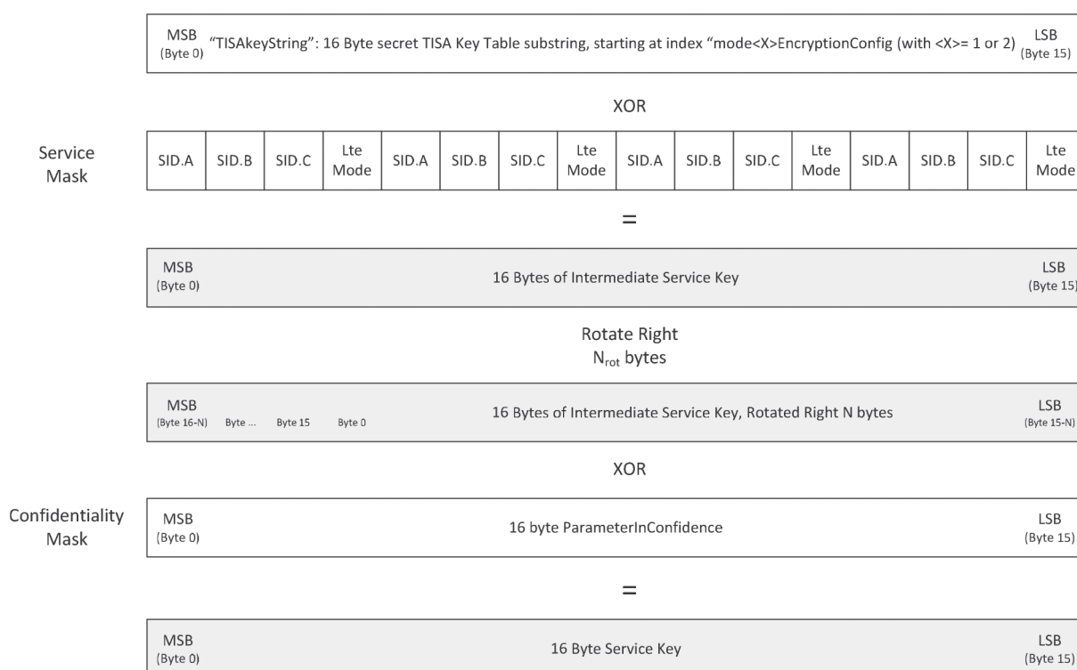
Figure 5 — Procedure for composing a Service Key, based on the secret TISA Key Table, transmitted service parameters and the ParameterInConfidence
