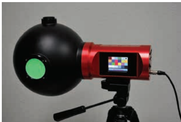
Figure A.1 — Sample of integrating sphere emitting bluish green light
