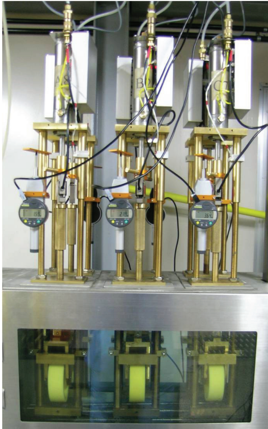
Figure A.5 — Pneumatically actuated notched ring loading device with electronic displacement gauge assembly
