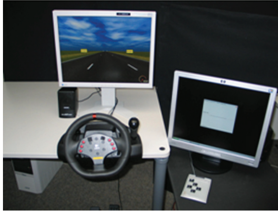
Figure A.2 — Setup for primary task (LCT example) and secondary task (CTT example)
