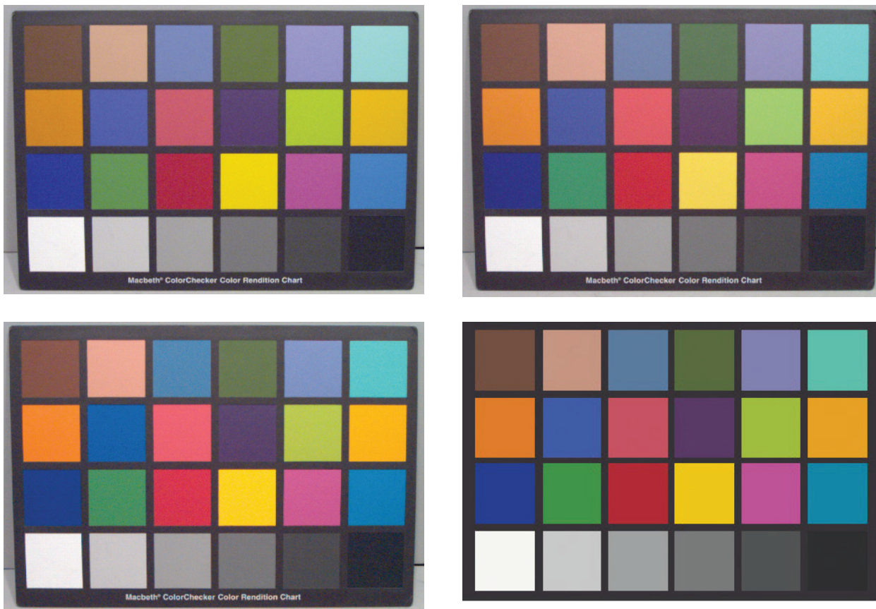
Figure 2 — Scene-referred images of a Macbeth ColourChecker™ 1) produced from the same raw image data but using different scene analysis transforms
