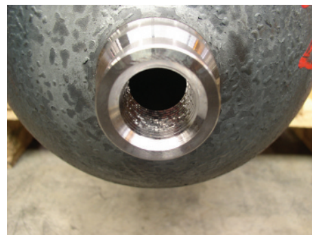
Figure A.14 — Chipped thread
