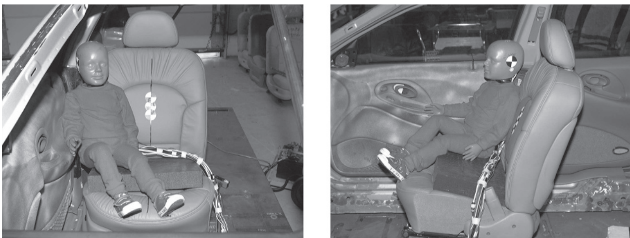
Figure 1 — Three-year-old-child on booster seat facing forward leaning against the door trim panel
