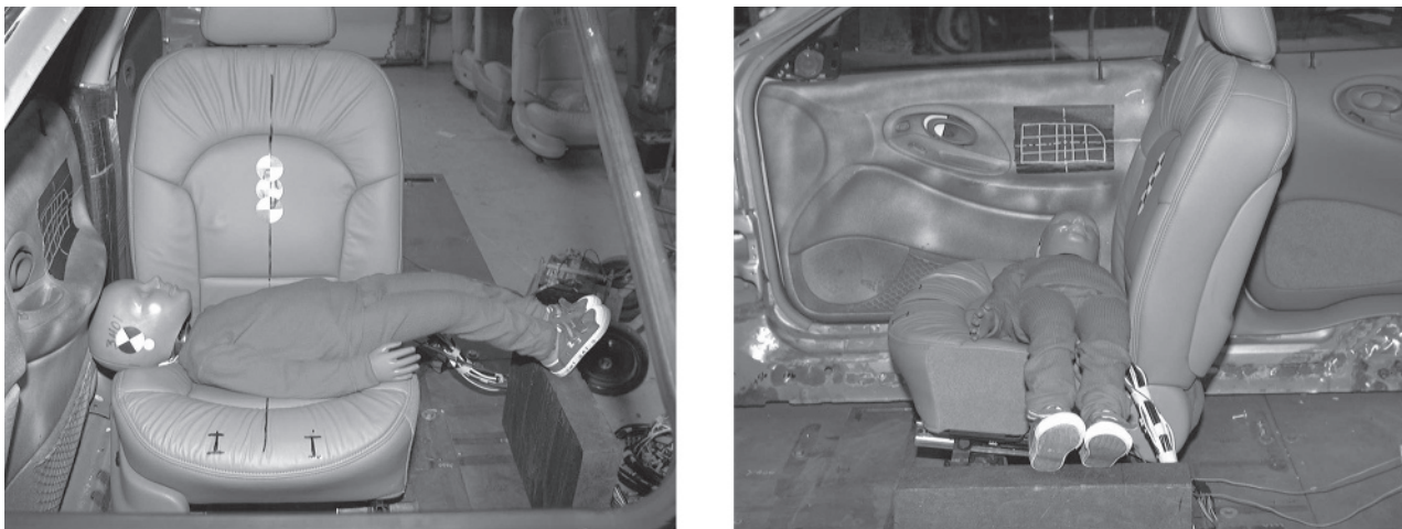
Figure 8 — Child lying across seat with head against the door trim panel (door/quarter-mounted air bag system)
