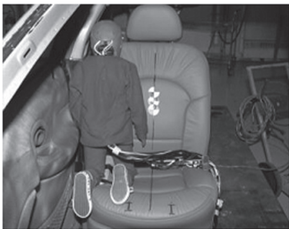
Figure 4 — Child facing rearward in vehicle leaning against door — High bolster-type seat (illustrated by foam taped to bolster)
