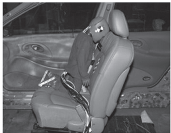
Figure 4 — Child facing rearward in vehicle leaning against door — High bolster-type seat (illustrated by foam taped to bolster)
