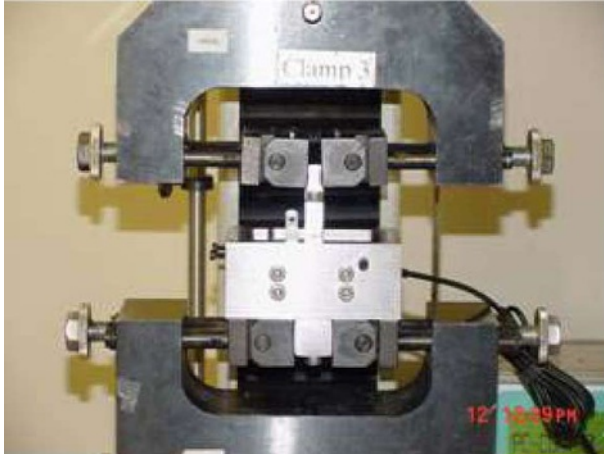
Figure D.1 — Fixture during rip-off force test
