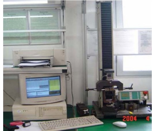
Figure D.2 — Machine for rip-off force
