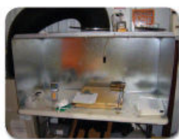
Enclosing hood with HEPA exhaust constructed to control possible emission of nylon nanofibers during destructive testing.
