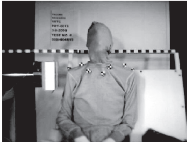
Figure B.2 — Impactor test configuration from the lateral shoulder impacts conducted by OSU (front view)[3],[4]
