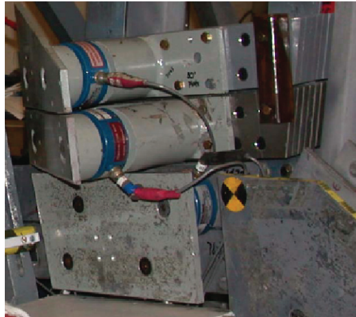
Figure F.3 — Impact wall configuration from the lateral sled tests conducted by MCW for the angled thorax and abdomen plate tests (forward oblique view)[41]
