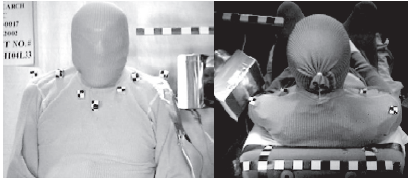
Figure B.4 — Impactor test configuration from the oblique-lateral shoulder impacts conducted by OSU[4] (frontal and overhead views of a 30° impact to the left shoulder of a PMHS)
