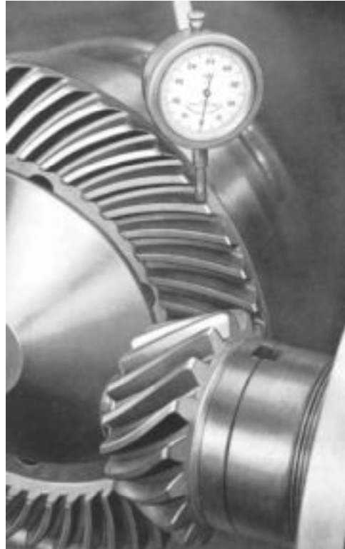
Figure 26 — Measurement of backlash in a pair of gears by means of a dial indicator
