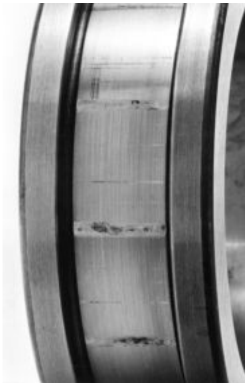
Figure 26 — False brinelling on inner ring raceway of cylindrical roller bearing
