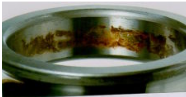
Figure 25 — Fretting corrosion in inner ring bore
