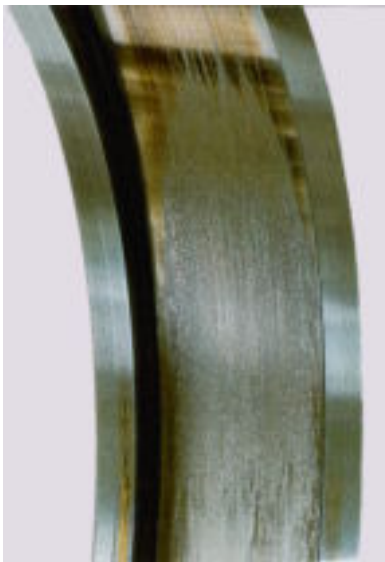
Figure 19 — Smearing on raceway surfaces
