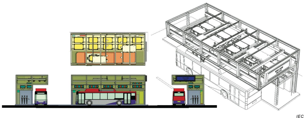
Figure B.2 – Automatic top-swapping station layout
