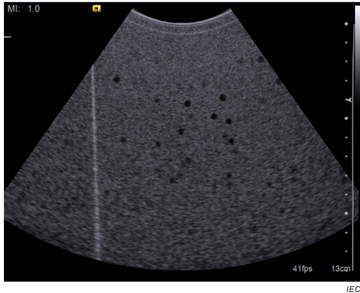
Figure B.1 – Convex-array image of a prototype 4 mm-diameter low-echo sphere phantom for use in the 2 MHz to 7 MHz frequency range
