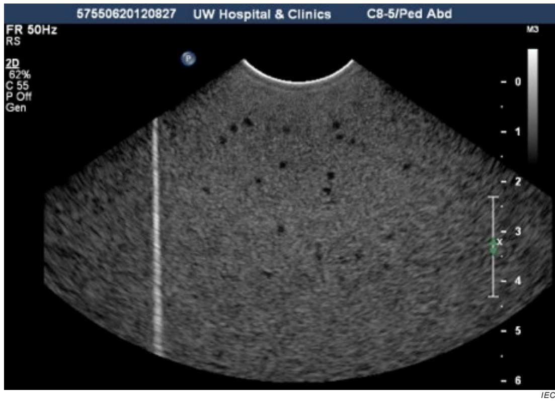
Figure D.2 – Image obtained by using the phantom containing 2 mm-diameter, low-echo spheres and a pediatric transducer with a radius of curvature of about 1,5 cm
