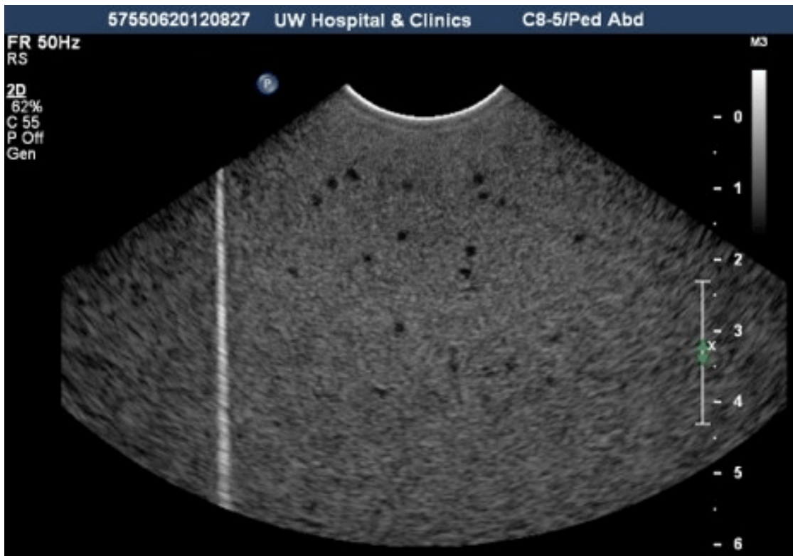
Figure C.8 – Image of the phantom containing 2 mm-diameter, low-echo spheres, made with a curved array having 1,5 cm radius of curvature, with its focus at 3 cm
