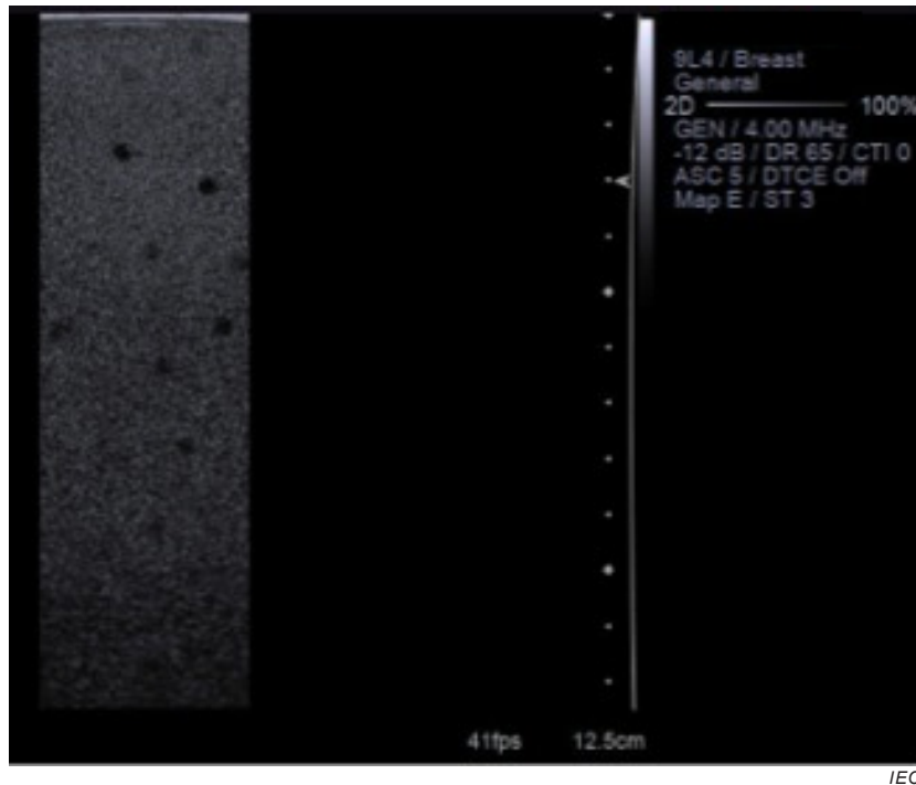
Figure B.5 – One of 80 parallel linear-array images of the phantom containing 4 mm-diameter, low-echo spheres, at 4 MHz with focus at 3 cm
