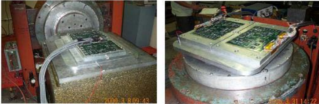
Figure C.5 – Mechanical shock test set-up 7
