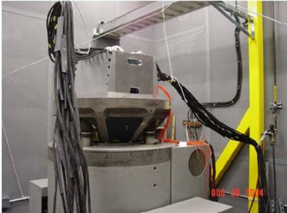
Figure C.3 – Vibration table showing Y-axis 6
