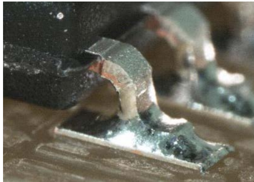
Figure B.1 – Insufficient solder flow
