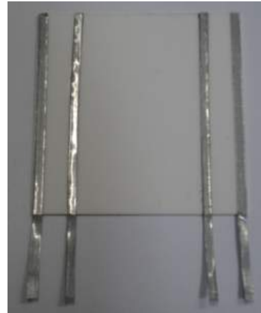
b) Alumina substrate with metal collector strips
