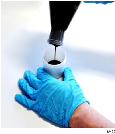
a) Electrode casting slurry
