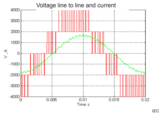
Figure A.11 – Three level topology with nominal voltage of maximum 2 400 V and timescale of 5 ms/div
