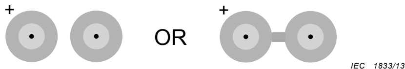
Figure 8a – Single or multi-conductor cable where each conductor is both insulated and sheathed
