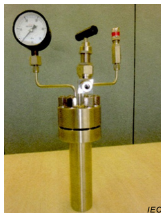
Figure 1 – Autoclave example for ageing test of EIM
