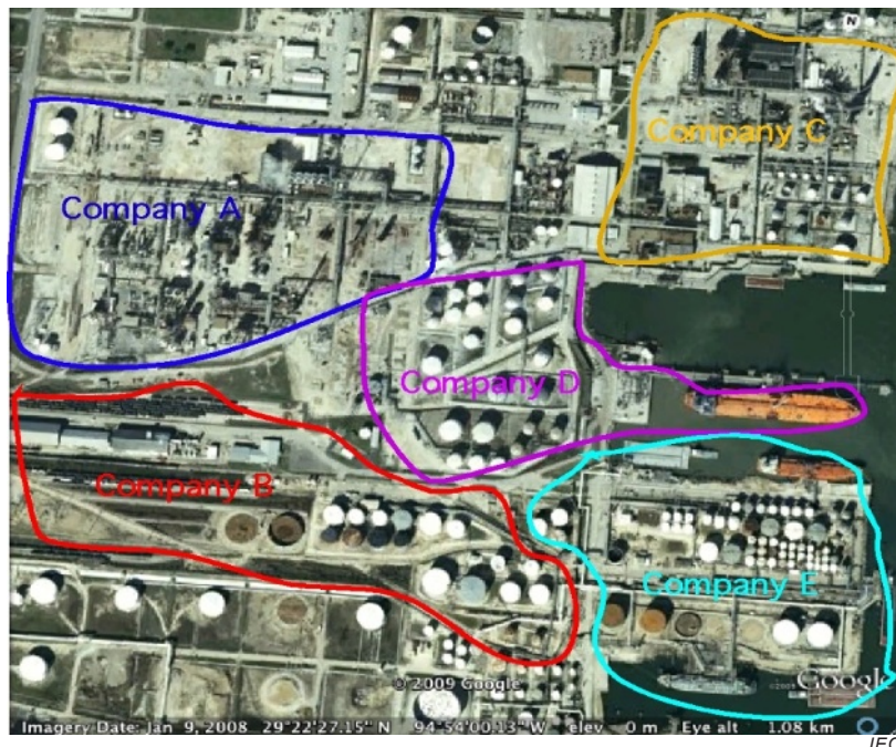
Figure B.13 – Networks deployed at neighbouring facilities will not “cross-talk” if non-routing nodes are deployed along the periphery of each facility
