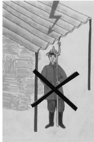
Figure 4 – Unsuitability of metallic structures when not earthed
