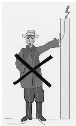
Figure 5 – Electrization by touch voltage
