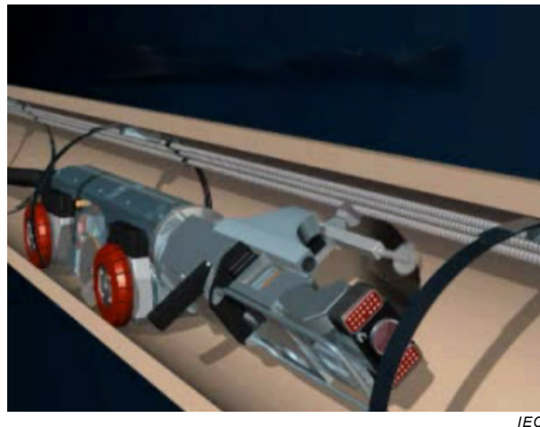
Figure 16 – Conduit robotized installation
