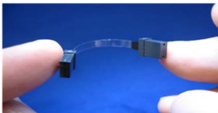
Figure 6c- Flexible optical circuit board using optical waveguides
