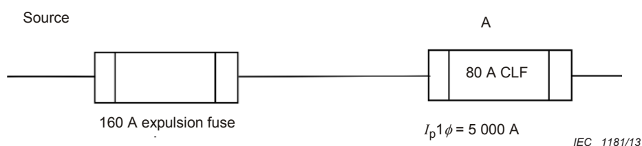
Figure 17 – Expulsion fuse/Current-limiting fuse example
