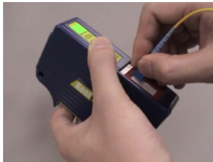
Figure 7 – Cleaning with a reel type cleaner
