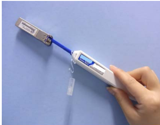
Figure C.2 – Cleaning optical transceiver receptacle end-face using a pen type cleaner
