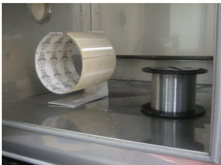
Figure 3 – Example of a possible set-up in temperature cycling
