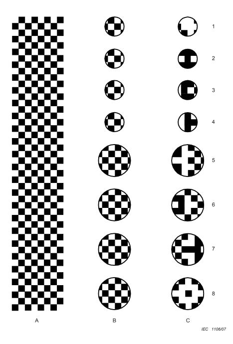
Figure 2 – Examples of circular disc test pieces according to 4.2.13.3
