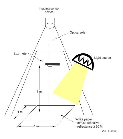
Figure 3 - Lux measurement setup at indirect light tests
