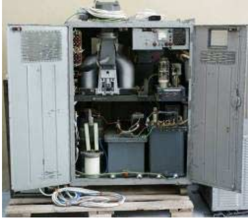
HPM generator 3 GHz
