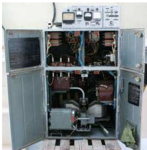
HPM generator 6 GHz
