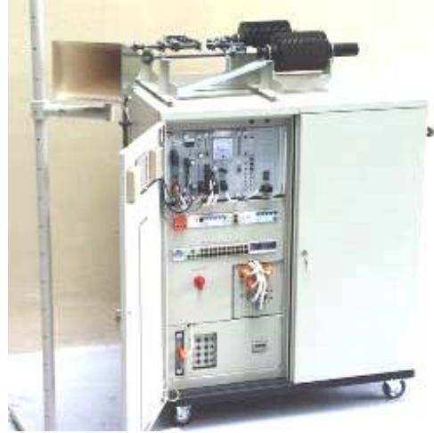
HPM generator 9 GHz with antenna 3 dB beam angle = 10°
