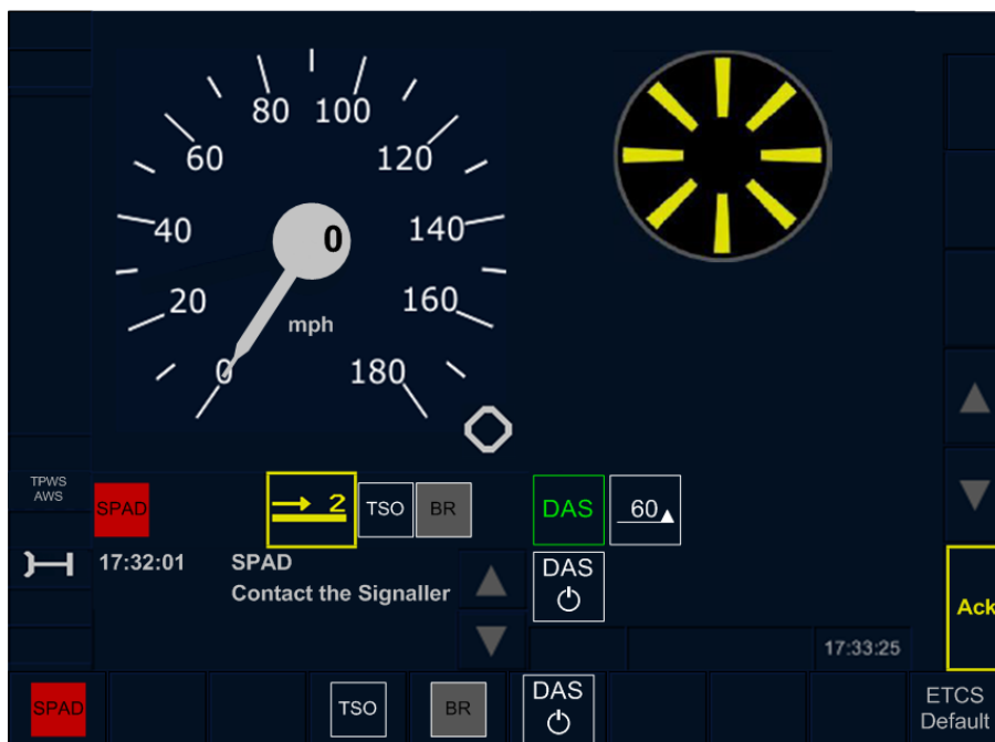
Figure A.11 — ETCS and AWS/TPWS window in soft key technology
