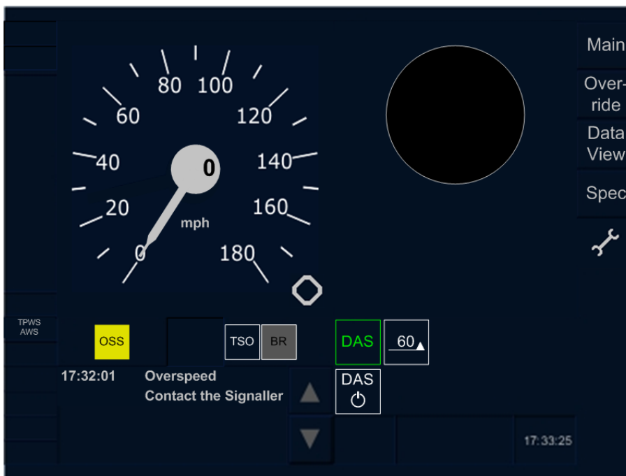
Figure A.12 — AWS/TPWS window in touch screen technology
