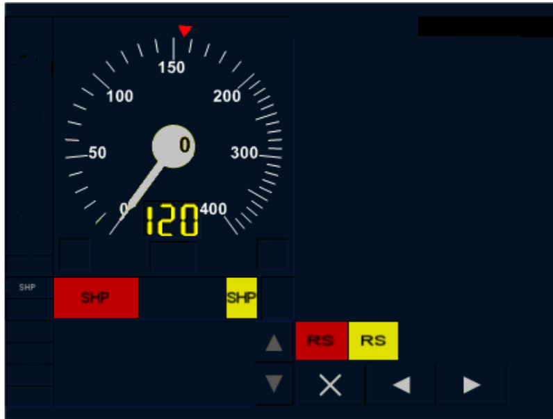
Figure A.29 — SHP default window in touch screen technology
