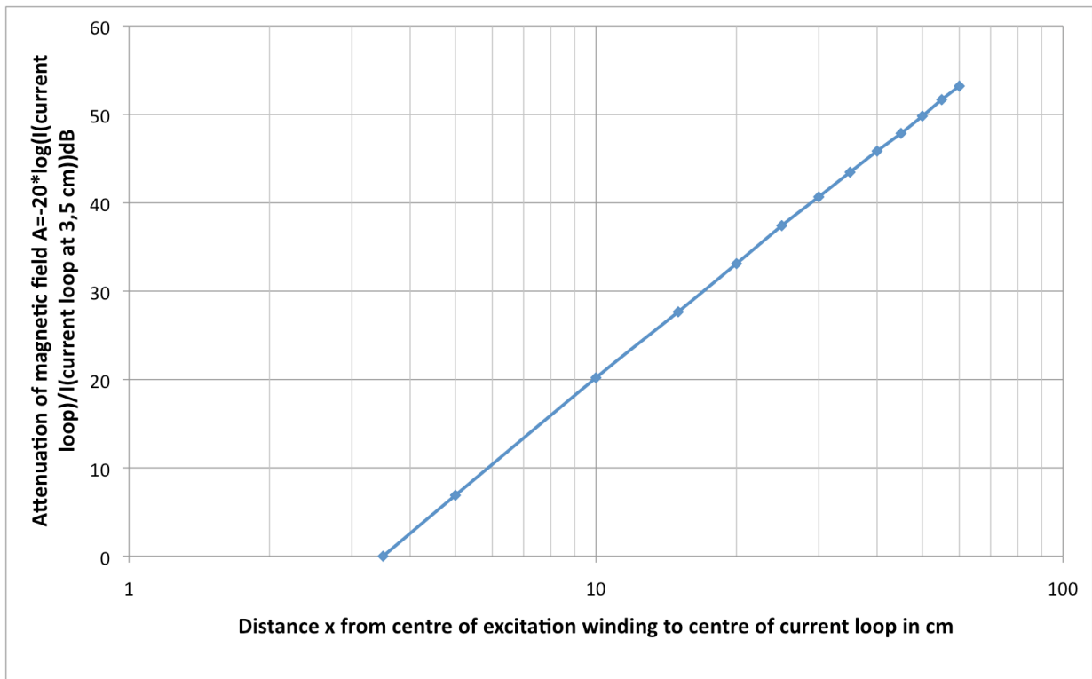
Figure A.3— Variation of the magnetic field with the distance to a perturbing power cable
