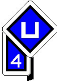
Figure 12 — End of neutral section
