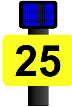
Figure 43 — Point work identification
