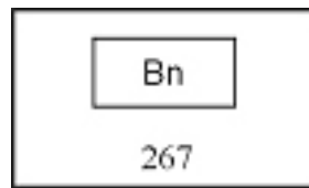
Figure 94 — Commencement of station area
