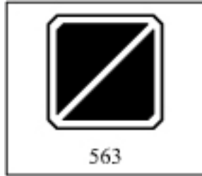
Figure 92 — Missing distant signal
