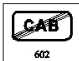
Figure 91 — Termination of cab signal area
