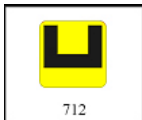
Figure 101 — End of neutral section
