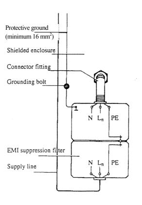
Figure 2 - Filter installations schematic
