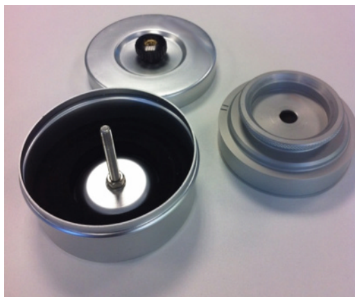
Figure 4 — The drum and its protection box [Source: RNSA]
