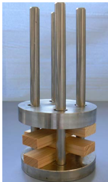
Figure 3 — Example of a holder to load the specimens
