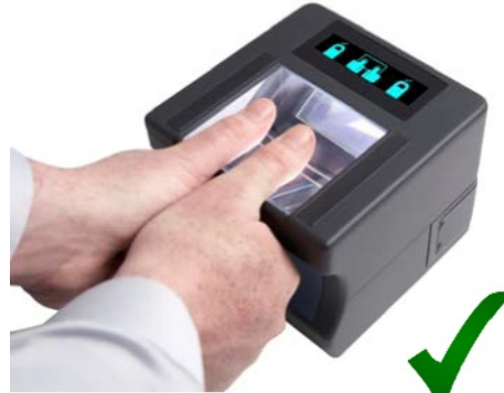
Figure 16 — Thumbs correct placement
