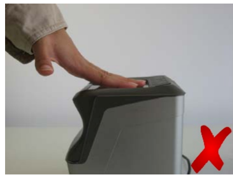
Figure 14 — Oblique pressure on the sensor
