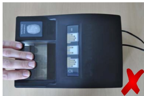
Figure 9.b — Mind the low border of the sensor
