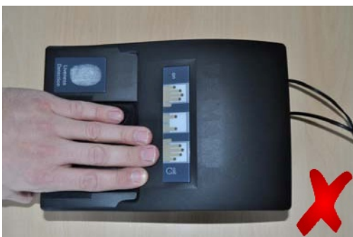
Figure 9.a — Mind the top border of the sensor
