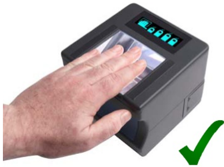
Figure 15 — Fingers correct placement
