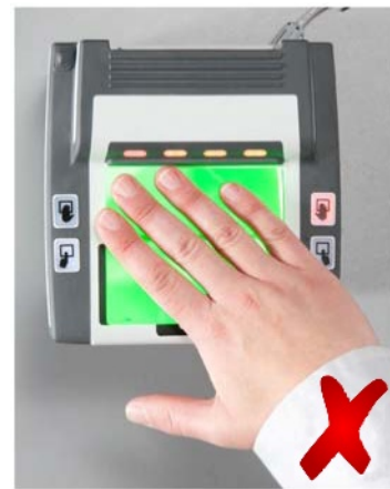
Figure 4 — Avoid rotated fingers in relation to the edges
