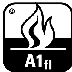
Figure 16 — Reaction to fire - Class A1 fl
