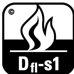
Figure 23 — Reaction to fire - Class D fl -s1
