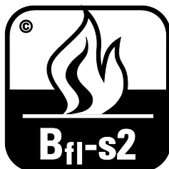
Figure 20 — Reaction to fire - Class B fl -s2
