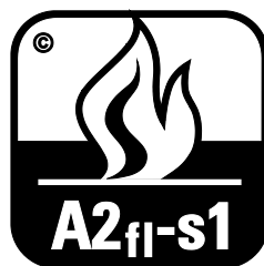
Figure 17 — Reaction to fire - Class A2 fl -s1
