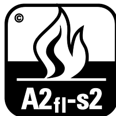
Figure 18 — Reaction to fire - Class A2 fl -s2
