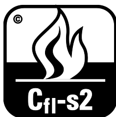
Figure 22 — Reaction to fire - Class C fl -s2
