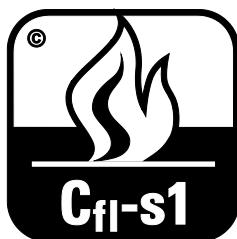
Figure 21 — Reaction to fire - Class C fl -s1
