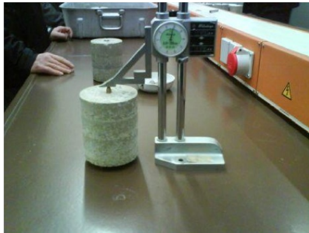
Figure A.3 — Demonstration of height measurement
